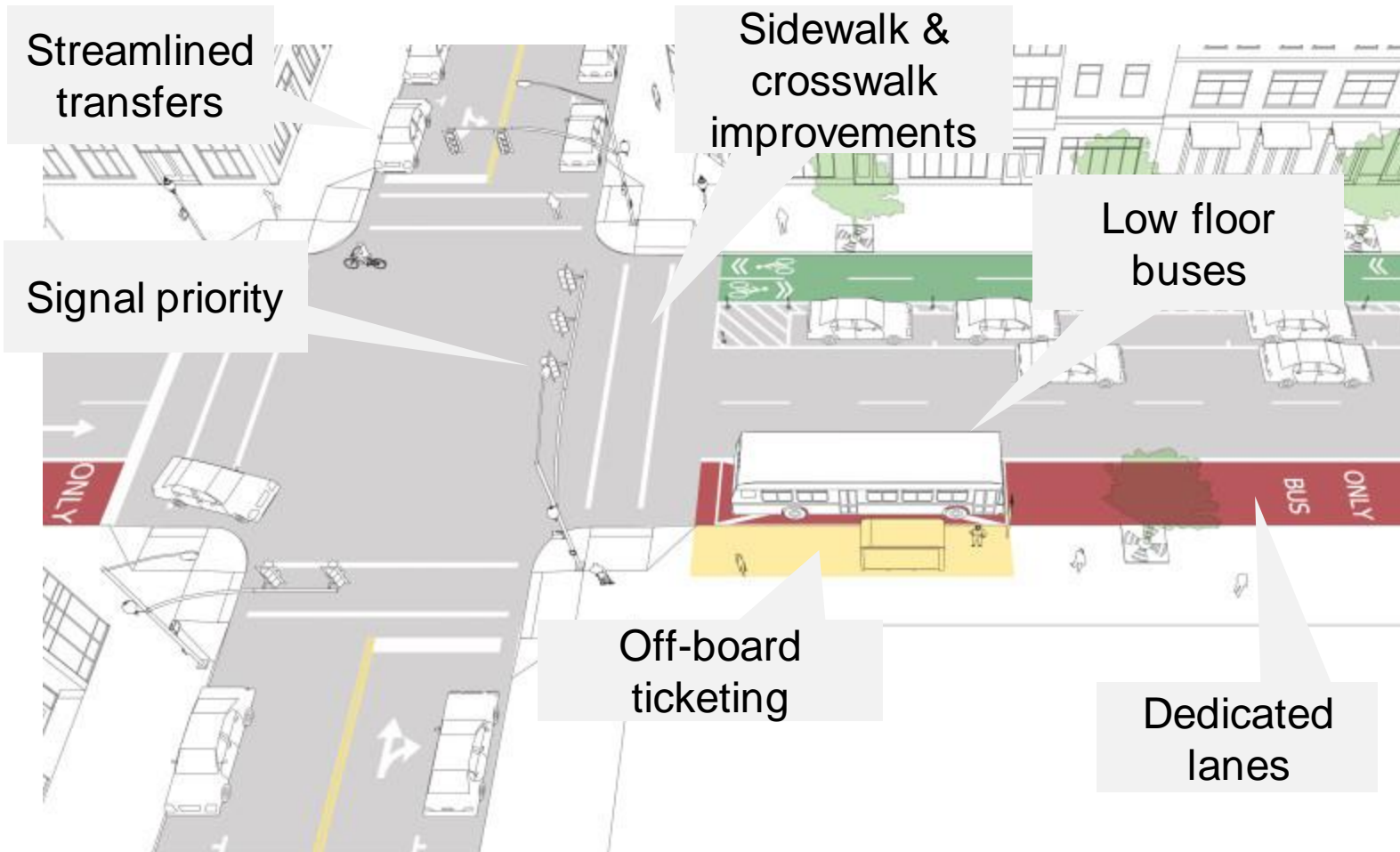
Image description: This is an illustration of an urban intersection showing various features of Bus Rapid Transit, including dedicated lanes and prioritized traffic signals. Source: NACTO
